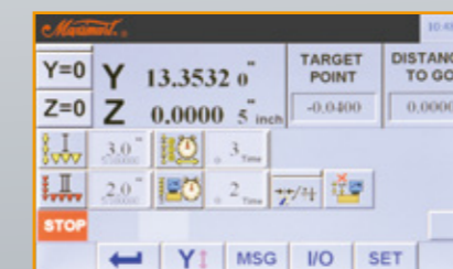
NC Downfeed page (Rough grinding / Finish grinding / Sparkout setting) Minimum display unit: Y-axis: 0.001 mm, Z-axis: 0.001 mm
