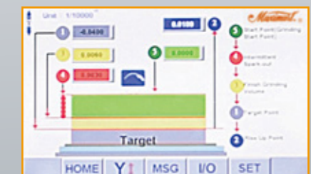
NC Setting of the grinding value
